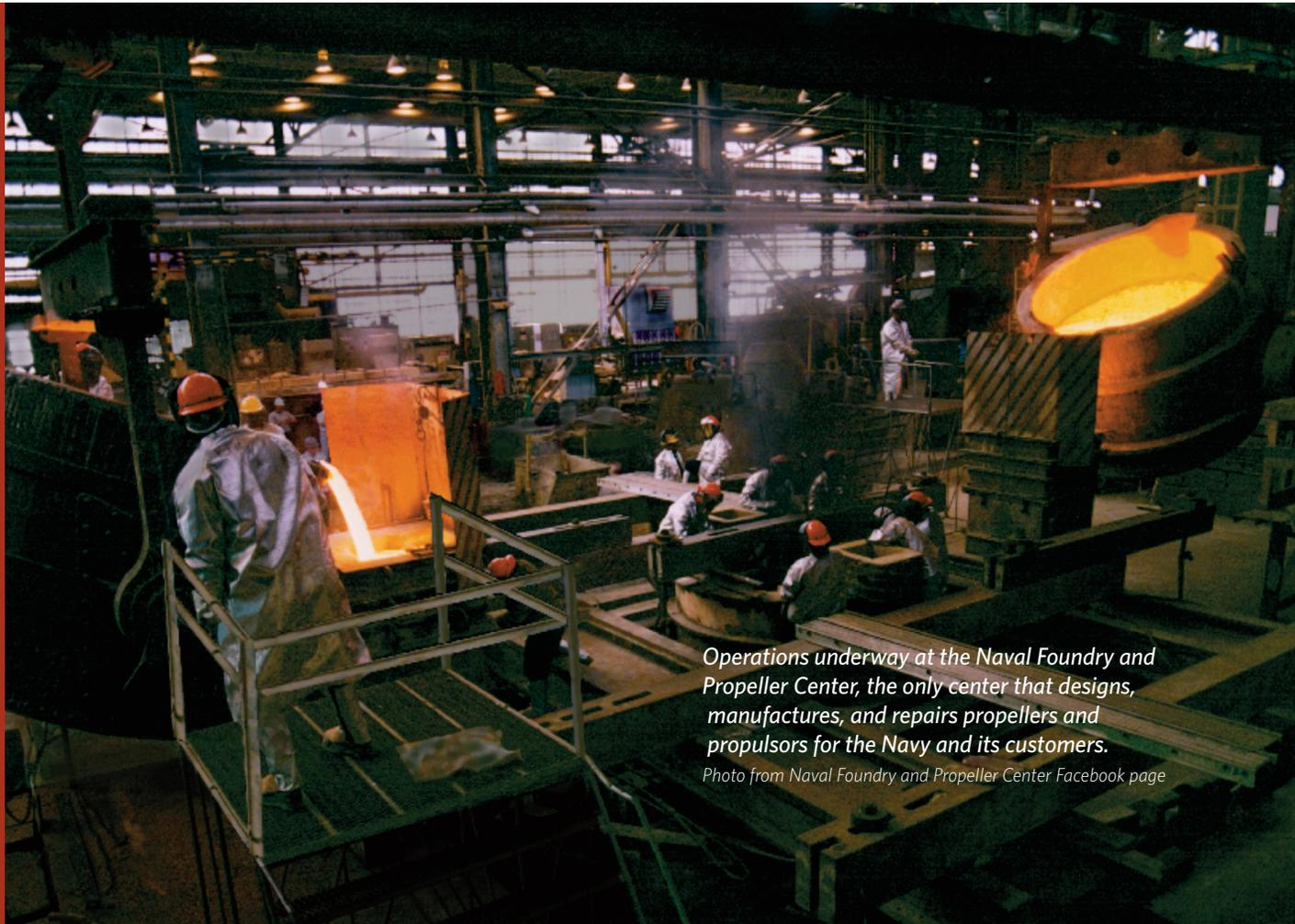
*Operations underway at the Naval Foundry and Propeller Center, the only center that designs, manufactures, and repairs propellers and propulsors for the Navy and its customers.*
